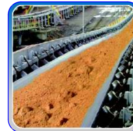
Steelcord/Sempercord (steelcord belt as per DIN)
